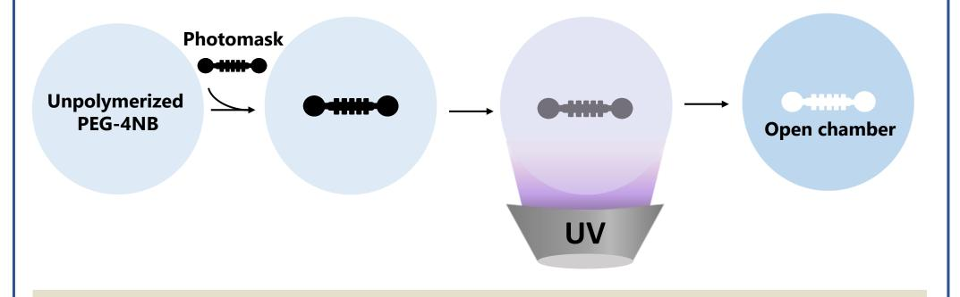
Photopatterning of complex structures in synthetic hydrogels, including perfusable channels for cell culture and media perfusion, in less than 1 second
