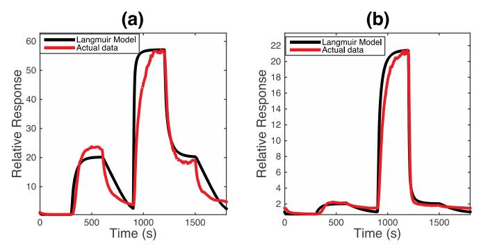
Response (red) of p-type (a)  $PSi/TiO_2$  (b)  $PSi/Au_xO$  interfaces to 5ppm of NO (0 s - 300 s), NH<sub>3</sub> (900 s - 1200 s) and NO + NH<sub>3</sub> simultaneously (300 s - 600 s and 1200 s - 1500 s) compared to the simulated (black) response. Note that the response of the mixed gas levels off to a specific value independent of which gas was first exposed to the sensor.
