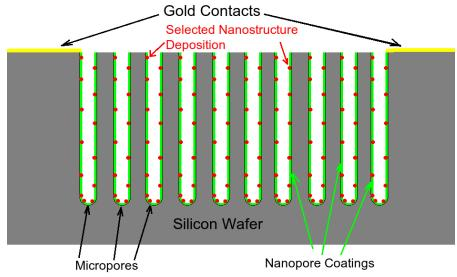
\*Nanostructured sites easily accessed- Fickian diffusion and rapid analytenanostructure interaction greatly improve micropore sensitivity.
