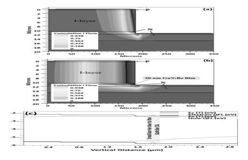
These figures show a pin diode structure having: (a) 10 ?m UID GaN i-layer and (b) 10 ?m GaN:Be i-layer and 50 nm GaN:Be thin film sandwiched in the n-type GaN layer. Current uniformity is improved from ~40% in (a) to ~100% in (b). Figure (c) is an energy band diagram of (b) for a 1 ?m i-layer under forward bias indicating a small energy barrier introduced by the thin GaN:Be current spreading layer.
