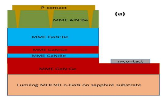
Layer structure diagram of quasi-vertical AIN JBS diode that uses intentionally cracked layers to form periodic JBS structures.
