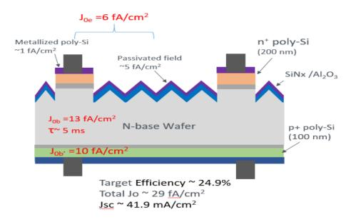
An example double-side TOPCon solar cell structure and efficiency
