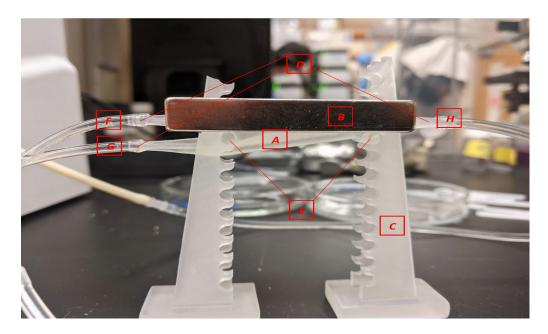
The magnetophoretic separator device, including (A) main separation chamber, (B) permanent magnets, (C) stand, (D) tapered connectors for flexible tubing, (E) mounting pegs, (F) outlet for magnetic material, (G) outlet for non-magnetic material, and (H) inlet.
