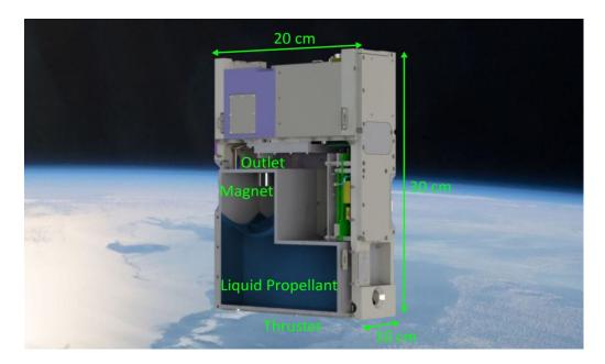
Conceptual representation of a magnetic positive positioning system on a CubeSat platform
