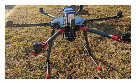
Georgia Tech Research Institute (GTRI) researchers used this UAV to flight test Distributed PNT Chain techniques developed to provide navigation support in the absence of GPS services. (Credit: GTRI)
