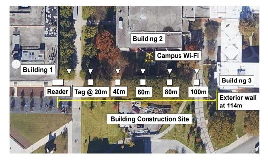
Top view photograph illustrating an experimental arrangement for measuring distance to prove accurate ranging in a realistic environment at more than 100 meters.
