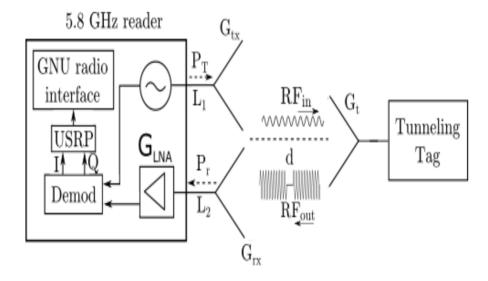
Schematic example of an RFID reader interrogating and receiving a modulated signal from a QTT.
