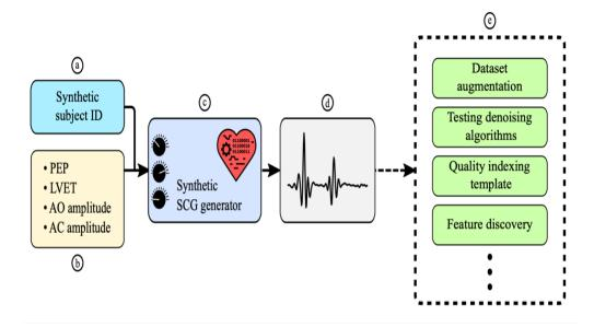
Overview of the synthetic SCG generator model. (a) A participant identification (ID) is fed as input, which controls the morphology of the generated beat. (b) The model receives SCG features as inputs and then outputs an SCG beat with those features. (c, d) This model can be used to generate sequences with controlled features. € This enables tasks such as dataset augmentation and template generation. It also sets the stage for simulating noisy SCG and testing denoising algorithms.
