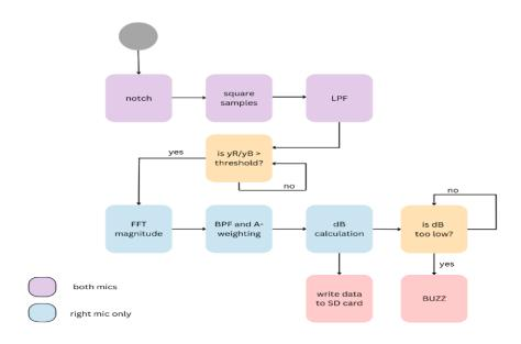
Flow chart of the Speech Assisting Multi-Microphone System (SAMMS) device with haptic feedback.
