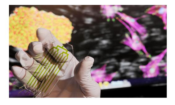
Close-up view of the microfluidic device that exploits the differences in adhesion strength between derived stem cells and contaminating cell types in a heterogeneous culture to selectively isolate cells of interest using fluid shear forces. Credit: Gary Meek
