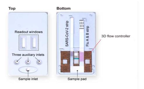
The device fully assembled in the 3D-printed case (left) and with its front cover removed (right). The back cover holds the internal components: commercial LFA strips of SARS-CoV-2 and influenza A and B and the paint-programmed paper-based flow controller.
