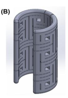
The auxetic-patterned implantable device of 2-mm wall thickness, showing different line widths and intervals.
