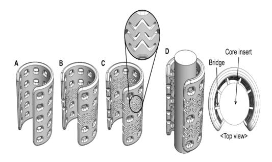
Design of the airway scaffolds. (A) Airway scaffold without stent-pattern. (B) Airway scaffold with a stent-pattern. (C) Airway scaffold with two stent-patterns. (D) The two stent-patterned airway scaffold with the core insert to create the tubular tissue flap *in vivo*.
