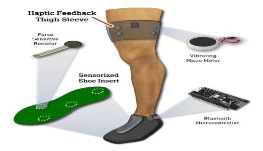
Foot-ankle orthosis with flexible sensory insole and fitted sleeve with discreet haptic feedback built-in.
