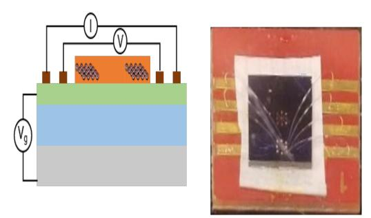
(Left) Device concept showing current (I), voltage (V), and gate voltage (Vg). (Right) Early device prototype. (Further development focuses on developing methods for additive manufacture of the devices [e.g., inkjet printing].)
