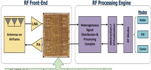
TRAFFIC: Software reconfigurable dynamic front-end analog processor for tunable filtering, linearization and compensation, interference mitigation, signal rejection, etc. ... before digital conversion and processing
