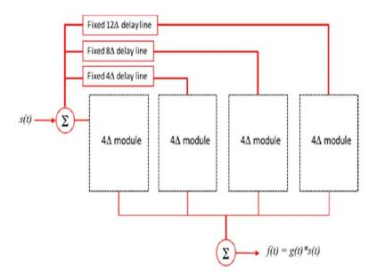
Modular analog TRAFFIC architecture that uses a series of small multi-tap (~4 taps) transversal filters.
