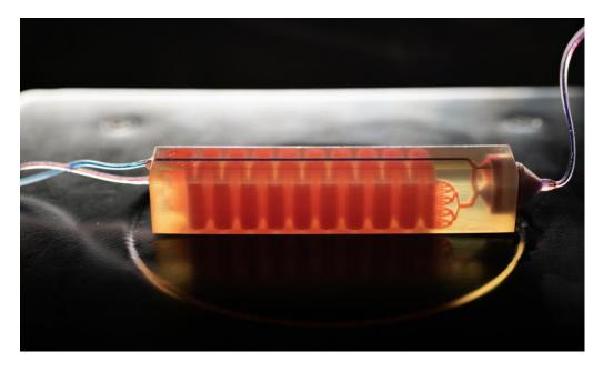
A 3D-printed cell trap developed in the laboratory of Georgia Tech Assistant Professor A. Fatih Sarioglu captures blood cells to isolate tumor cells from a blood sample. (Photo: Allison Carter, Georgia Tech)
