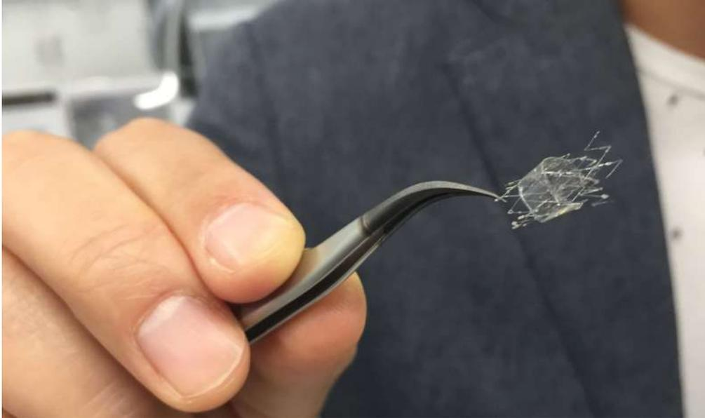
A flow sensor is shown here on a stent backbone. Credit: John Toon, Georgia Tech
