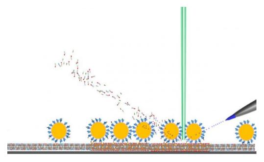
BeamMap uses an electron beam to image topology, provide localized heating to promote desorption and allow precise determination of the location of the spray capillary and electrospray impact area for imaging. The electrosprayed liquid beam at a controlled energy level is used to desorb and charge analytes for chemical imaging in BeamMap.
