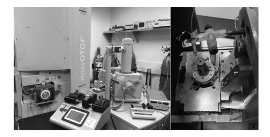
Image shows a mass spectrometer and scanning electronic microscope that provide the foundation for the BeamMap system, which can simultaneously determine surface topology and chemical makeup of a biological sample.
