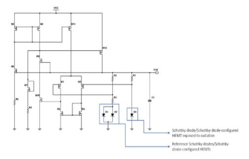
This figure represents the bandgap reference circuit for Georgia Tech's semiconductor particle detector.
