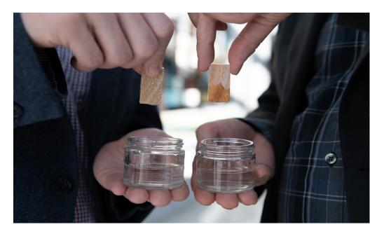
Treated (left) and untreated (right) pieces of lumber after being submerged in water. The treated wood resists absorbing water while the untreated wood readily soaks it up, causing a color change in seconds.
