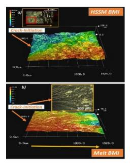
These images compare roughness qualities in both an HSSM BMI and a simple melt BMI at a crack initiation zone.
