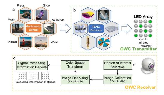
An illustration of the self-powered OWC system that includes (a) the potential mechanical stimuli that can be monitored, (b) different TENG devices working with the LED transmitter, and (c) the OWC receiver that detects the information conveyed by the light
