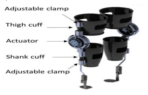
Georgia Tech's powered bilateral knee exoskeleton features a lightweight, low-cost, low-profile assembly weighing only 1.5 kg and a single-stage actuator for high back drivability.
