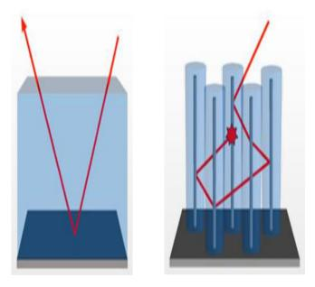
Traditional planar PVs (left) allow for only a single impingement of the photon, which limits absorption. Antireflection (AR) coatings can improve upon this deficiency but only to a limited extent due to wavelength dependency of the AR coating. Georgia Tech's CNT-based textured device (right) permits multiple wavelengthindependent impingements of a single photon, which significantly increases absorption probability.
