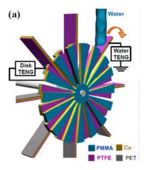
This hybridized TENG includes disk-TENG and water-TENG to harvest both aspects of mechanical energy. The TENG's material components include poly(methyl methacrylate)
