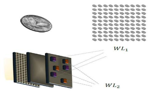
Neuro-inspired computing platform and associated architecture composed of microchips with arrays of weak learners (WLs) used in decision-making tasks that may be implemented in electronic, photonic, or other engineering platforms
