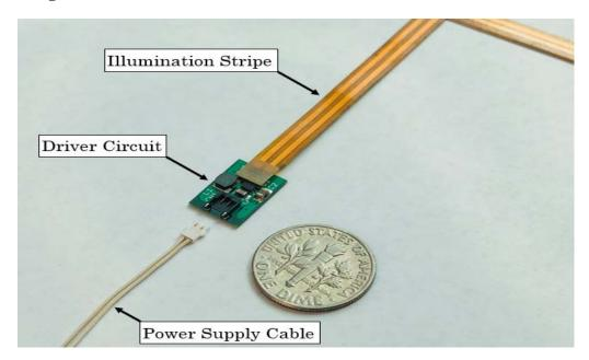
The systemâ??s small-form driver circuit and illumination stripe connecting to the power supply
