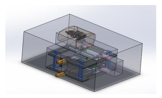
Proposed validation setup for the 5DOF MRE actuator positioning system, tissue mimicking phantom fixed above the MRE actuator, with both the robot and phantom set into a low-density foam block.
