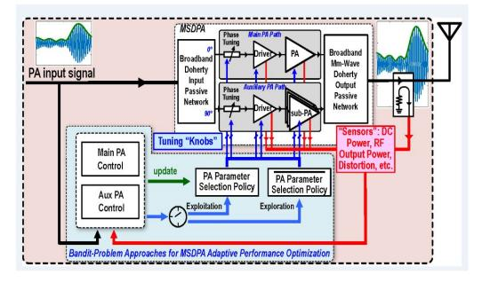
Conceptual diagram of the AI-assisted mm-wave Doherty PA. The mixed-signal Doherty PA (MSDPA) contains main and auxiliary PA paths. Both inputs and the sensed outputs are sent to the control unit, which runs RL-based algorithms to achieve extended linear gain region while maintaining high PA efficiency.
