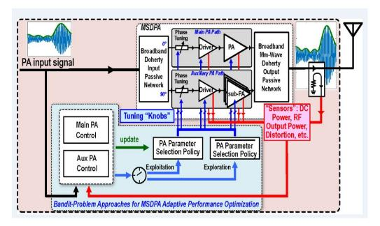
Conceptual diagram of the AI-assisted mm-wave Doherty PA. The mixed-signal Doherty PA (MSDPA) contains main and auxiliary PA paths. Both inputs and the sensed outputs are sent to the control unit, which runs RL-based algorithms to achieve extended linear gain region while maintaining high PA efficiency.
