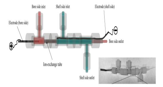
Tubular design of the power module.
