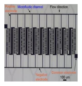
A diagram of the microfluidic device with 10 code-multiplexed Coulter sensors, each with a unique sensor signal
