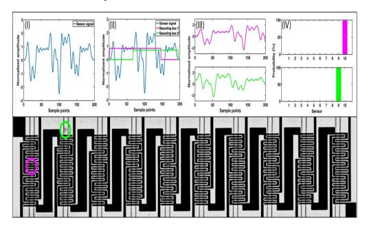
ConvNet decoding process of a sensor waveform with simultaneously-recorded high-speed camera image.
