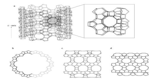
Construction of the nanotube shown only in tetrahedral atoms, built from an outer and inner layer
