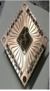
Prototypes of capillary trap and vapor pump thermal management devices
