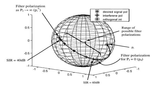
This is a graphical representation of weight vector polarizations for one OFDM sub-channel with signal-to-interference ratio levels ranging from approximately 60 dB to approximately 40 dB in approximately 5 dB steps.
