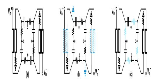
(a) A simplified schematic of Georgia Tech's dual-band quadrature signal generation network. (b) At low frequencies, the transmission lines of the coupled-line couplers are ideally short-circuited. (c) At high frequencies, the capacitances of the polyphase filters are ideally short-circuited.
