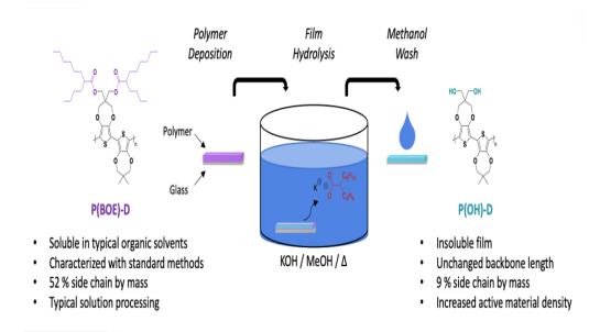
An overview of the film hydrolysis used in Georgia Tech's method for post-processing side chain cleavage
