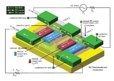
Diagram of the two-cell RF thermoelectric generator.
