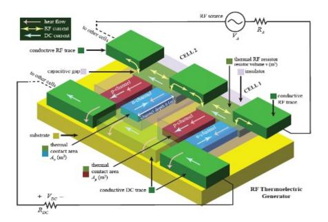
Diagram of the two-cell RF thermoelectric generator.
