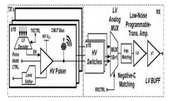
Simplified block diagram of the proposed architecture of the ultrasound receiver with the element-level impedance matching for low frame rate applications such as intracranial ultrasound
