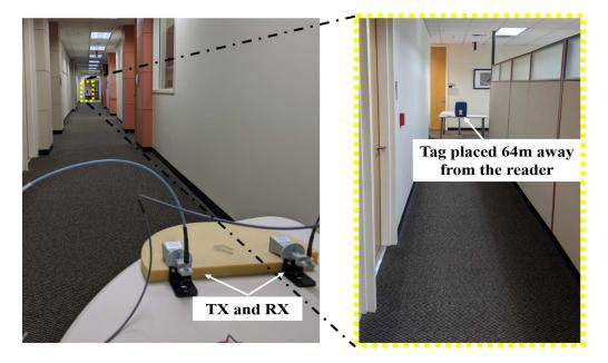
The setup and environment used to measure the Rotman lens-based tag's long-range capabilities
