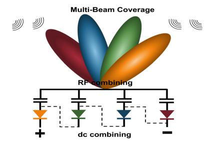
This technology enables dual combining (RF + DC) by the use of the Rotman lens between antennas and rectifiers.
