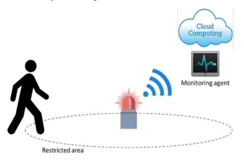
Sonar-based system for smaller work areas (e.g., lifting equipment, manhole inspection).
