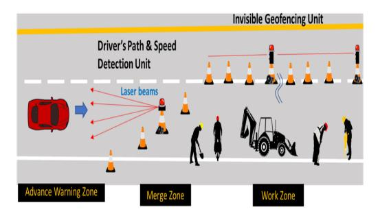
Lidar-based system for longer work zones
