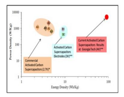
A comparison of commercial and experimental activated carbon-based supercapacitors.
