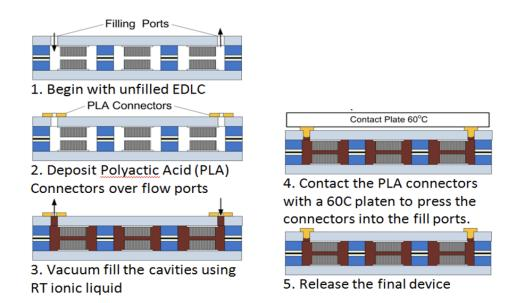
Baseline process flow for placing and sealing electrolyte within the micro-capacitor
