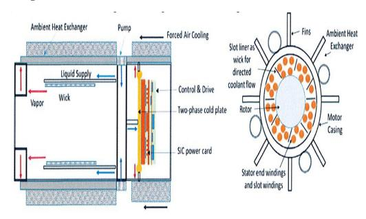
Georgia Tech's evaporative cooling system includes co-packaging of interior permanent magnet motor and wide bandgap electronics with embedded two-phase thermal management. A closed-loop, wick-assisted evaporative system provides cooling of stator windings (left). The motor cross-section (right) illustrates the windings and a possible configuration of the ambient heat exchanger.
