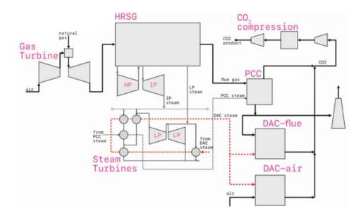
Simplified block diagram of the flexible power generation plant
