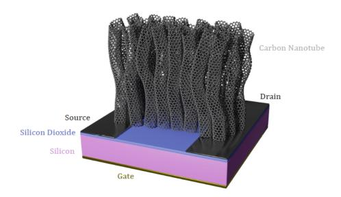
An illustration of Georgia Tech's vertically aligned CNT-based ionizing radiation detector.
