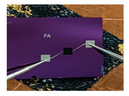
A fully fabricated detector with probing needles contacting electrode pads.
