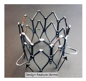
Georgia Techâ??s mechanism with arms extended. The arms must extend far enough to create a landing zone larger than the native annulus to allow for efficient THV deployment.
