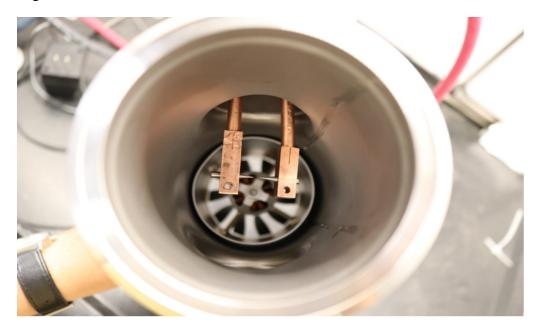
A demonstration system that allows researchers to test different electrode materials and geometries while characterizing the heat transfer into the high-speed airflow
