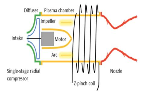
Single-stage radial compressor configuration showing the conceptual design for a small-scale demonstrator engine
