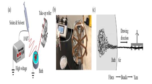
(A) Schematic of wet electrospinning; (B) Experimental setup of wet electrospinning; (C) Schematic of fabricating fibers, bundles, and yarns
