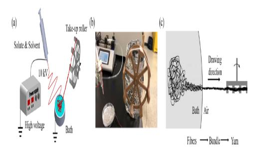
(A) Schematic of wet electrospinning; (B) Experimental setup of wet electrospinning; (C) Schematic of fabricating fibers, bundles, and yarns
